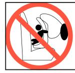
**WARNING:** DO NOT place a child restraint in the front seat of a vehicle with a passenger air bag unless the air bag is turned off. DEATH or SERIOUS INJURY can occur. The back seat is the safest place for children under 12.
