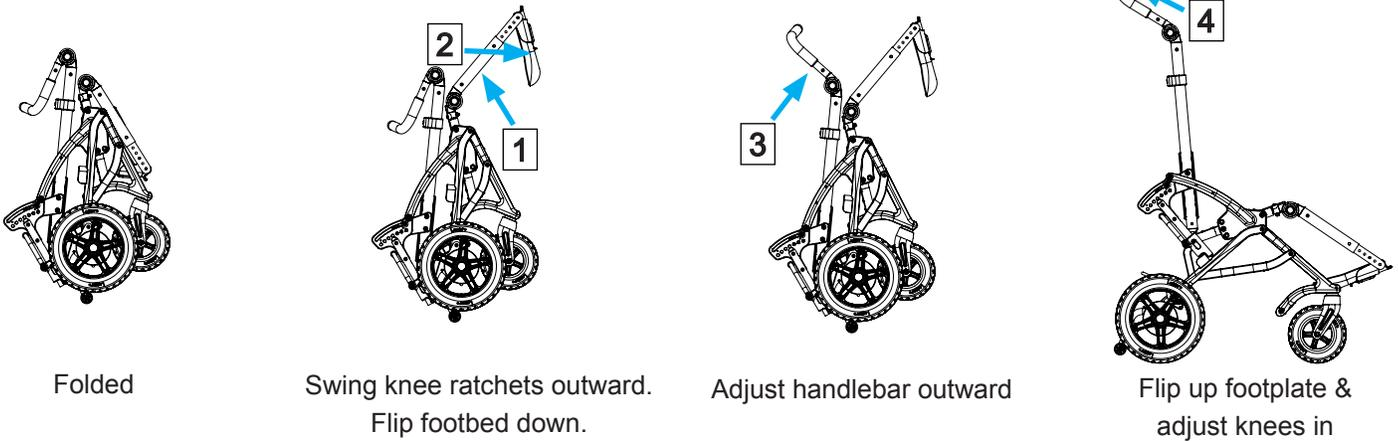
**WARNING!** When folding or unfolding, keep arms, hands, and feet clear of moving components to avoid injury. Reference Figure 13, arrows indicate potential pinch points.
