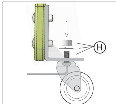
Install brake casters in the rear for stability. Use allen key to insert bolt up through the caster and bracket. Tighten nylon nuts with a crescent wrench. Note: Maintain tight screws.
