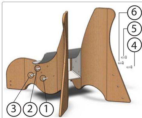
Attach (B) metal seat pan to (A) wooden sides with (6x) bolts. Install bolts in numeric order. Finger-tighten bolts until snug.
