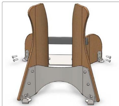
Attach (D) front brackets to (A) wooden sides with (4x) bolts. Finger tighten bolts first, then securely tighten with wrench. (Important : attach bracket to outside as shown)
