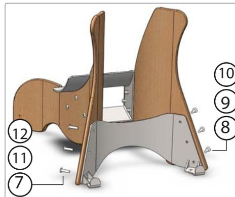
Attach (C) metal back bracket to (A) wooden sides with (6x) bolts. Finger tighten bolts first, then securely tighten the rear bracket bolts and seat pan bolts with wrench.
