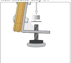
**04** Feed Non mobile glide up through base bracket. Install lock washers then nut. Note: Maintain tight screws.
