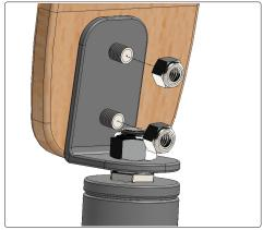
03 Be sure casters w/break are installed toward rear of base. This increases base strength. Maintain tight screws.
