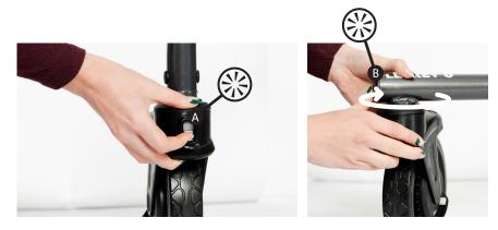
• Note – applying directional lock to all four castors will restrict the frame to a forward, straight-line direction only. Applying direction lock to both the rear castors will prevent excessive side-to-side movement of the frame by the user but still allows them the freedom to steer the frame.
