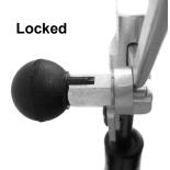
Pull and rotate pin 90° in the opposite direction to engage lock.
