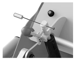
**A.** Position tilt piston axle midway through the tilt piston head.
