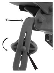
To adjust the footrest to desired height and angle, loosen round rubber knobs on both sides and reposition the Velcro. Tighten the round knobs to set the footrest position. To adjust the depth of the legrest extension, remove starshaped knobs and reposition to desired depth. Re-install the starshaped knobs.
