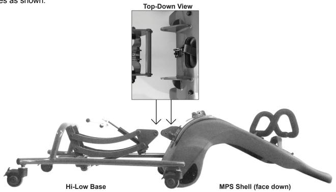
**B.** Install nylon spacers on Hi-Low mounting bracket.
