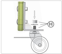
Install brake casters in the rear for stability. Use allen key to insert bolt up through the caster and bracket. Tighten nylon nuts with a crescent wrench. Note: Maintain tight screws.
