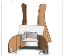
Attach (D) front brackets to (A) wooden sides with (4x) bolts. Finger tighten bolts first, then securely tighten with wrench. (Important: attach bracket to inside as shown)
