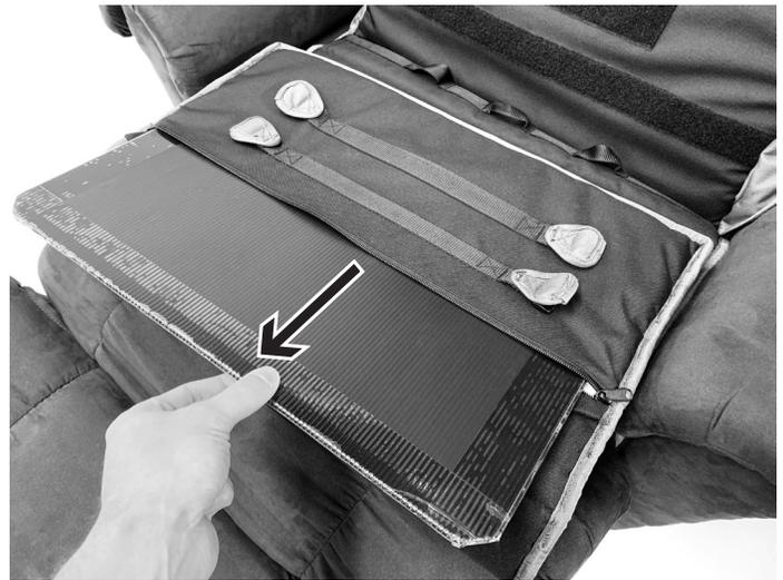
6. Re-install Fabric Liner Pad to Base Fabric.
